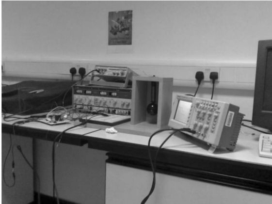
Fig. 2. Experimental setup built by students showing the magnetic levitation system, control board and instrumentation equipment.
