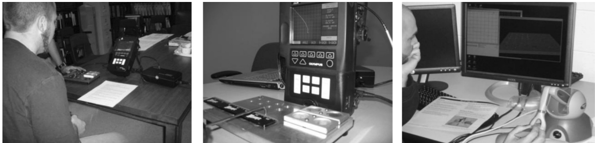
Fig. 3. User interaction with the actual eddy current simulator (left), graphical output (middle) and User interaction with Phantom Omni ® (right).
