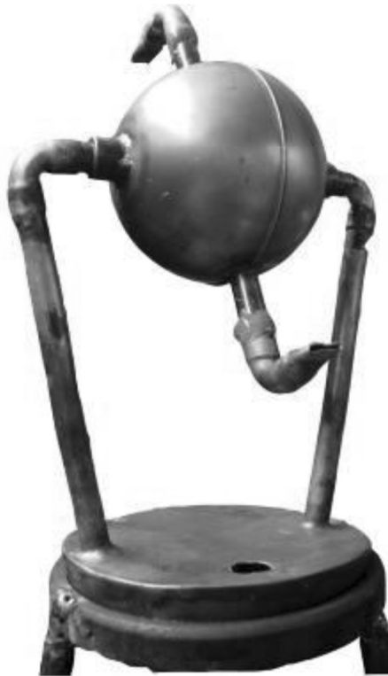
Fig. 3. Aeolipile presented at the Mechane contest.
