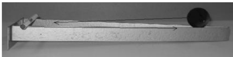
Fig. 1. The left side of the wedge above is elevated. The pen rolls 'down' along the edge towards the right. The double cone on the opposite end has an elevated center of mass when it rests on the narrower end (right side) of the wedge. When released, the double cone rolls left and 'sinks in' the wedge as it widens. This demo shows the pen 'falling to the right' while the cone 'falls to the left' which gives the illusion that the double cone is going up the incline.
