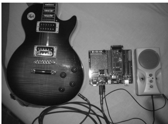
Fig. 5. The guitar effects pedal implemented in an FPGA.
