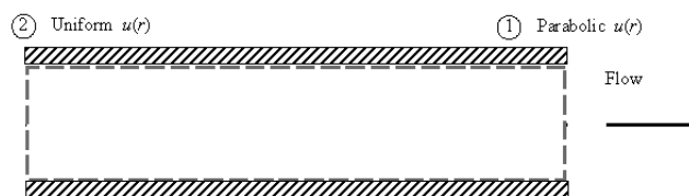
Fig. 6. Control volume selected to expose viscous frictional forces at the walls and pressure forces at the ends.
