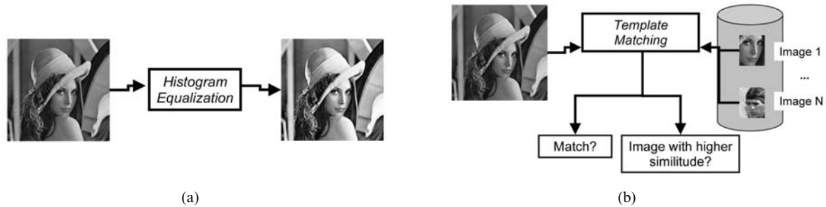
Fig. 4. Input/output results for two mini-projects: (a) image histogram equalizer; (b) image template matching.
