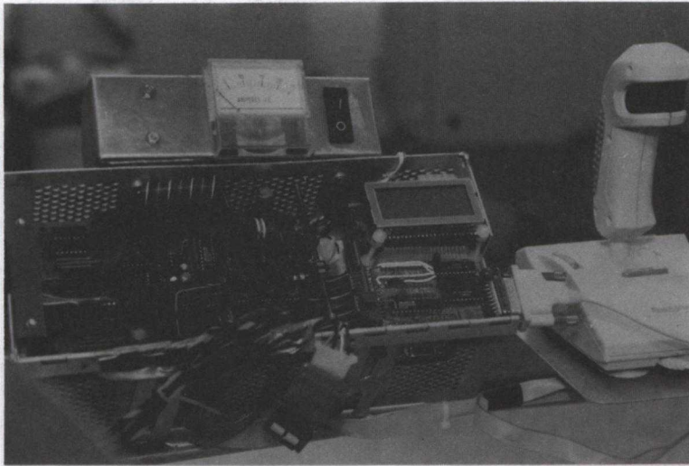
Fig. 10. Control hardware with display and operator's console.
