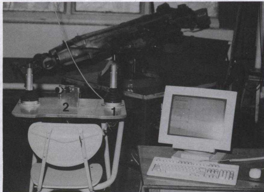
Fig. 3. General view of joystick-controlled hydraulic manipulator.
